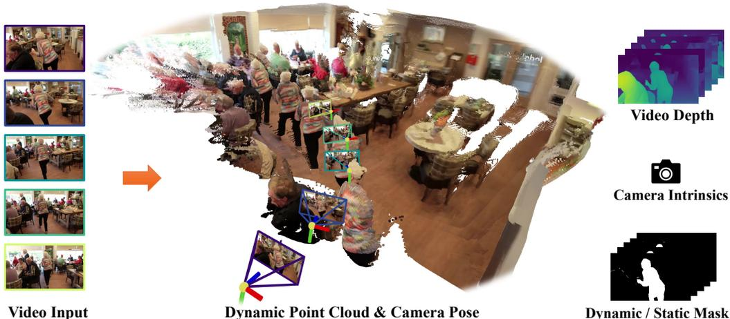
Figure 1: **MonST3R** processes a dynamic video to produce a time-varying dynamic point cloud, along with per-frame camera poses and intrinsics, in a predominantly feed-forward manner. This representation then enables the efficient computation of downstream tasks, such as video depth estimation and dynamic/static scene segmentation.
